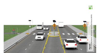
Rectangular Rapid Flashing Beacons
